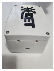
KET's HLPS box includes the valve that will be installed on the water supplying pipe in the room. The boxes will be installed throughout the hotel and data on water consumption will be sent via the segment in the box to a centralized unit where the water consumption can be monitored.
